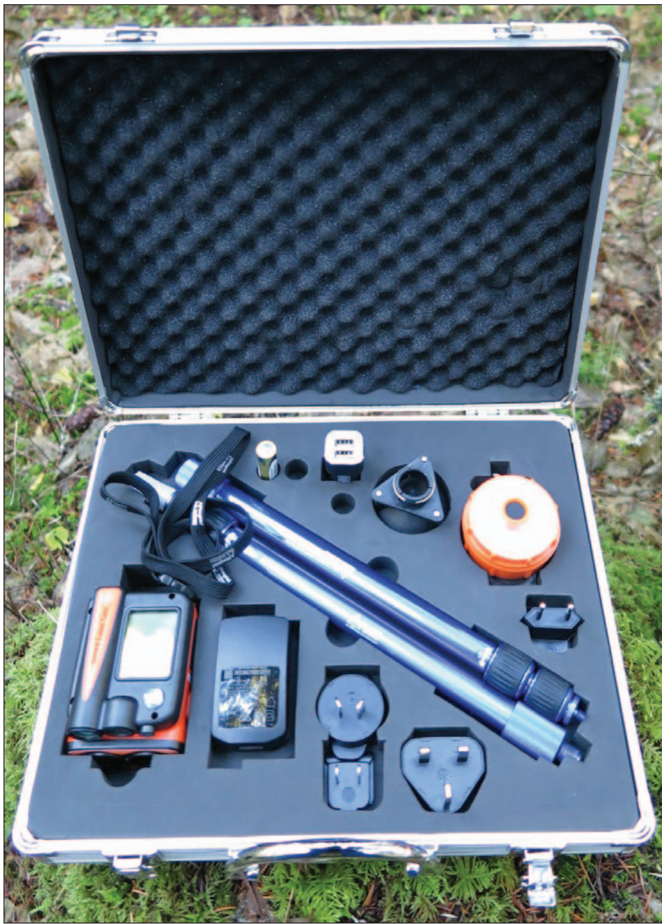
The Vertex Laser Geo with accessories in its carrying case.
