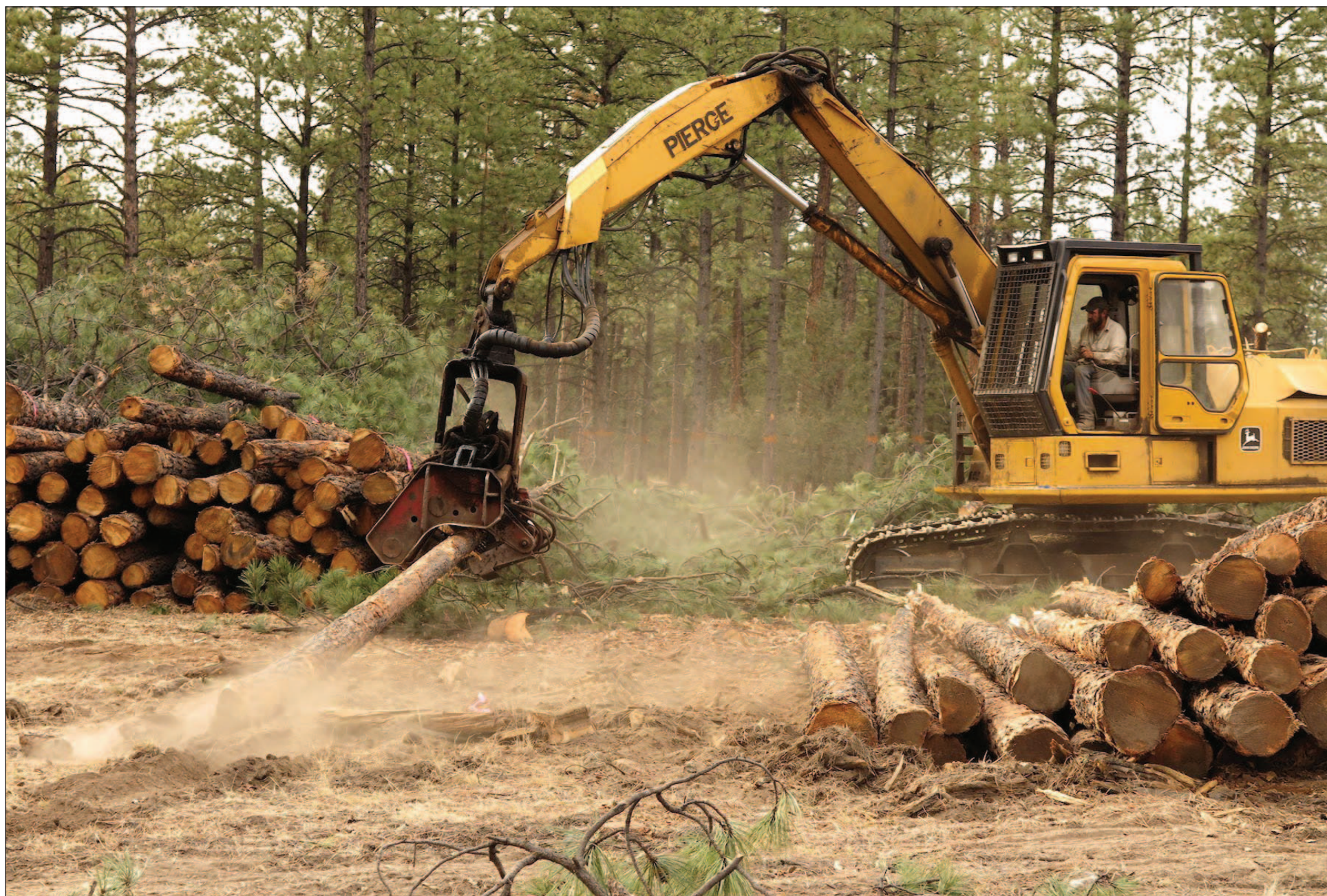
A delimitter processes ponderosa pine logs destined for Mt. Taylor Manufacturing, a sawmill in Milan, New Mexico, that produces dimension lumber, cants, wood pellets, playground chips, animal bedding, and other products.
