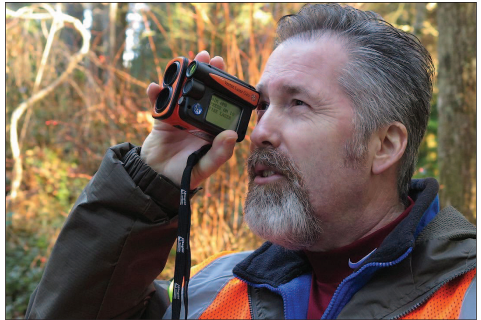
Haglöf's new Vertex Laser Geo: laser and ultrasound measurements, plus a GPS receiver and electronic compass. Photo by Steve Wilent.
